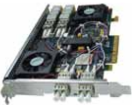
PE10G2DBI-SR: Dual port Fiber (SR) 10 Gigabit Ethernet PCI Express Content Director Server Adapter Intel® Based
